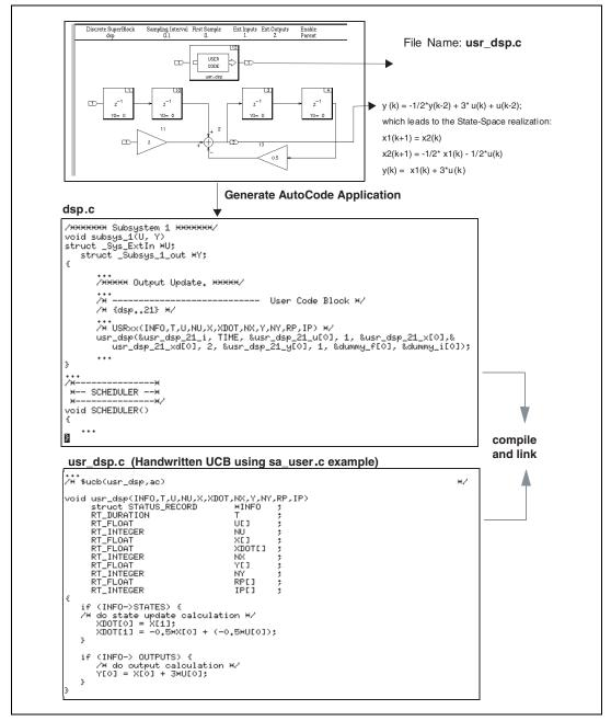
Figure 2-2. Linking Handwritten UCBs with AutoCode Applications
